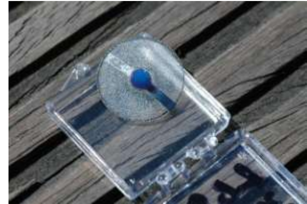
Diamond thickness shear mode resonator “nano balance”
